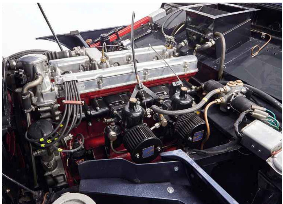
Right and opposite Forward-hinging ‘clamshell’ bonnet affords excellent access to the LB6 engine, though restoration specialists say it’s a devil of a job to achieve perfect shutlines when it’s closed. Bodies were originally made at the Tickford coachworks: although the early David Brown Astons are generally known as Feltham cars, in fact production had transferred to Newport Pagnell by the time of the MkIII’s launch in ‘57
